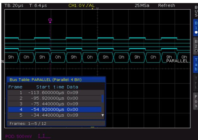
Fig. 13.3: Example PARALLEL BUS with BUS table
