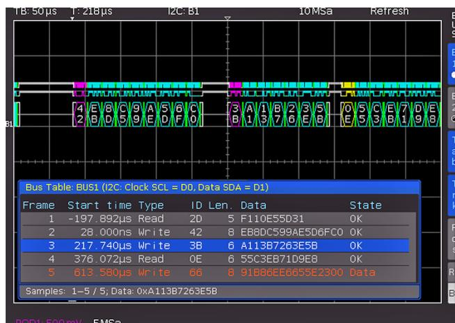
Fig. 13.2: Example I<sup>2</sup>C BUS with BUS table
