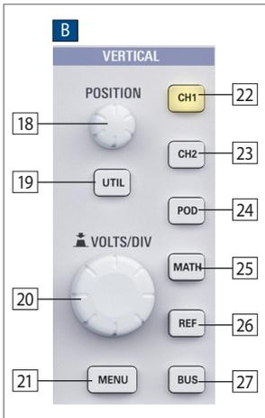
Fig. 4.1: Control panel for the vertical system
