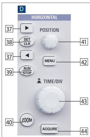
Fig. 5.1: Control panel of the horizontal system
