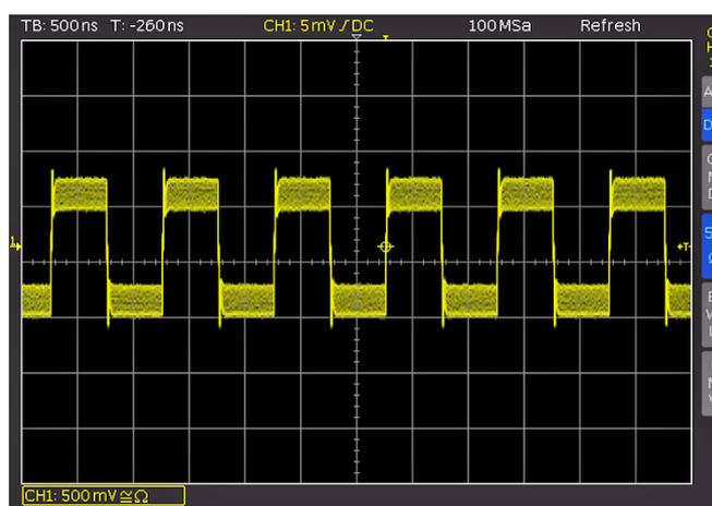
Fig. 5.2: AM modulated signal with maximum repeat rate
