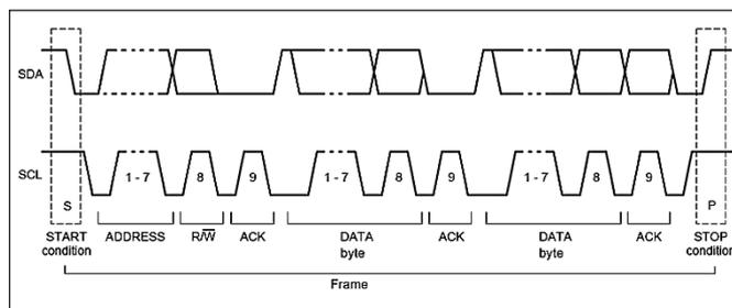
Fig. 13.4: I<sup>2</sup>C 7-Bit-Address
