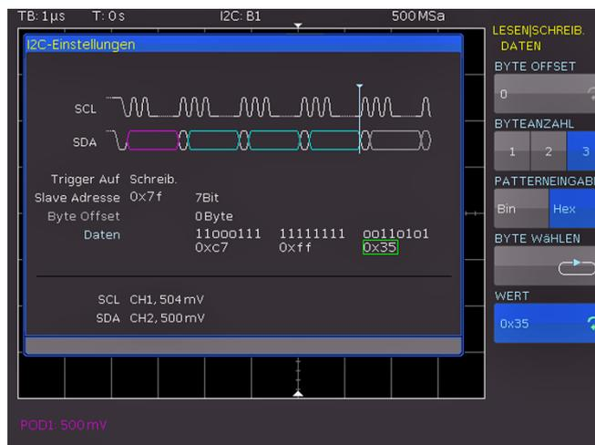
Fig. 13.5: I<sup>2</sup>C Read/Write trigger menu
