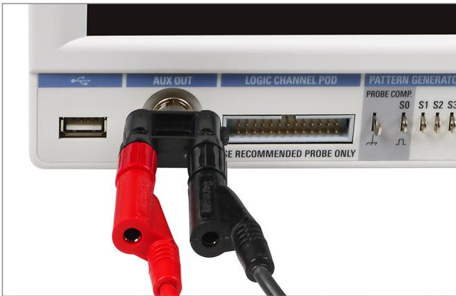
Fig. 9.9: HZ20 adapter connected to AUX OUT
