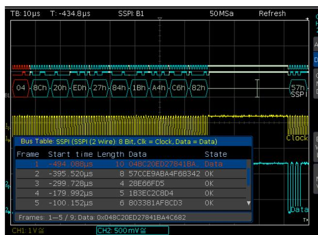
Fig. 13.10: Example SSPI BUS table
