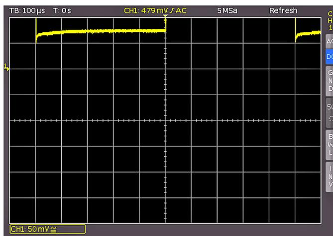
Fig. 3.3: Screen display after changing to DC coupling
