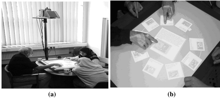
Fig. 10. (a) The Coffee Table, showing the video projector responsible for projecting information items onto the table surface. (b) Information items projected onto the surface of the Table move slowly around the perimeter. The interactive DiamondTouch surface (Ryall et al. [2004]) senses touch on a particular item which the coffee table software translates into manipulations of the information items.
